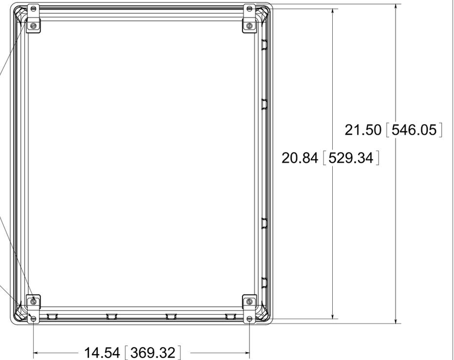
(4) EACH #10-32 BRASS INSERTS AND STAINLESS STEEL CAPTIVE COVER SCREWS WITH RETAINING O-RING
