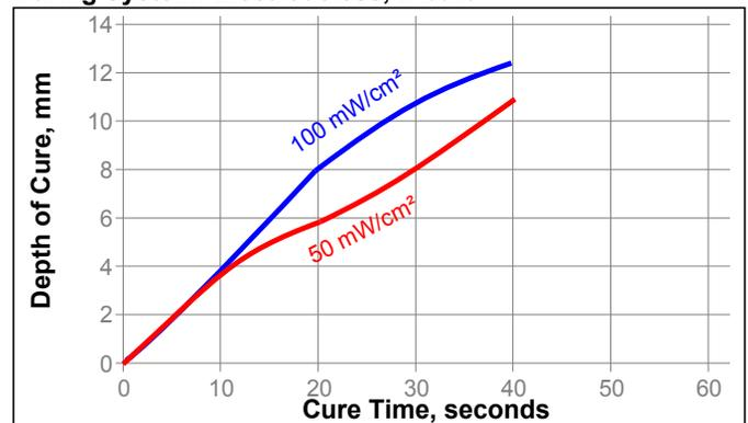
**Curing System: Electrodeless, H bulb**
