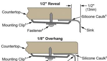
Designed to affix to the underside of any solid surface countertop.
