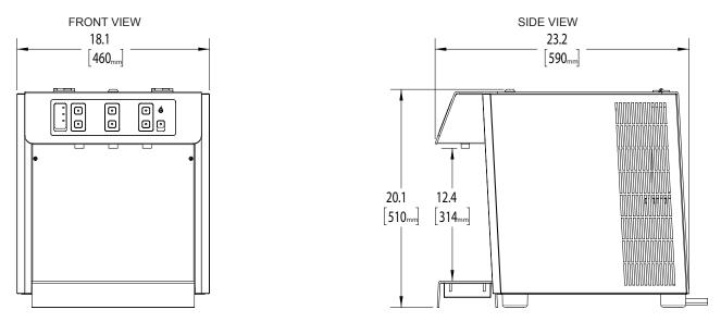
ELECTRICAL: 115 V -60 Hz. 1 Ph., 330 W – 3.2A, NEMA 5-15 Plug WATER SUPPLY: 3/8 in. supply recommended, 14.5 PSI min, 51 PSI max. (125 PSI max with use of supplied regulator) INSTALLATION: Provide 4 in. of clearance around unit to allow adequate ventilation **REQUIRES:**  $CO_2$  tank with standard threaded connection to CGA 320 nut,  $CO_2$  TANK IS NOT INCLUDED
