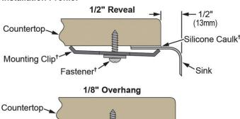
(3mm) †Not furnished Designed to affix to the underside of any solid surface countertop.
