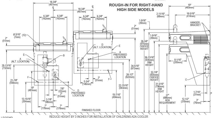
LEGEND A = Recommended water supply location. Shut off valve (not furnished) to accept 3/8" O.D. unplated copper tube connect. Up to 3" (76mm) maximum out from wall. B = Recommended waste outlet location. To accomodate 1-1/2" nominal drain. Drain stub 2" (51mm) out form wall.
