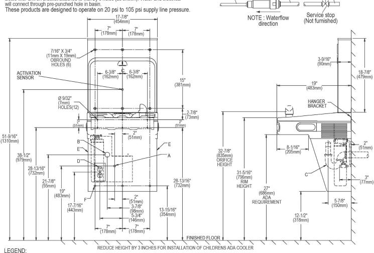
A = Recommended Water Supply location. Shut-off Valve (not furnished) to accept 3/8" O.D. unplated copper tube. Up to 3" (76mm) maximum out from wall. B = Recommended Waste Outlet location. To accommodate 1-1/4" nominal drain.
