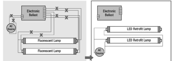
**FIG 3 - Retrofit with 2 Lamps**
