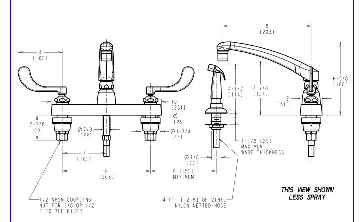
DIMENSIONS ARE IN INCHES AND [MILLIMETERS].
