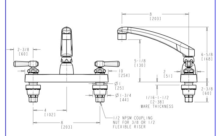
DIMENSIONS ARE IN INCHES AND [MILLIMETERS].
