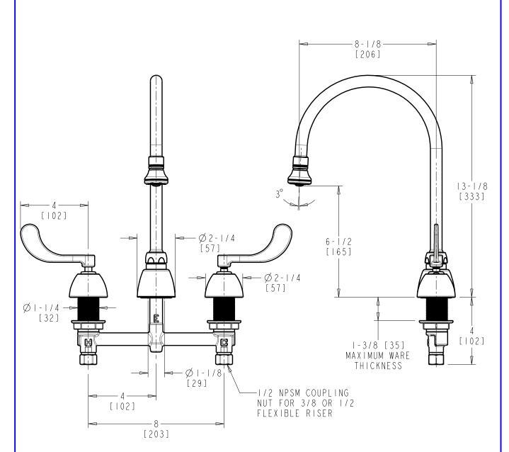
DIMENSIONS ARE IN INCHES AND [MILLIMETERS].
