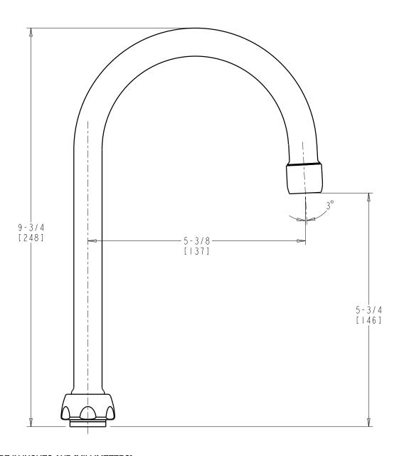
DIMENSIONS ARE IN INCHES AND [MILLIMETERS].
