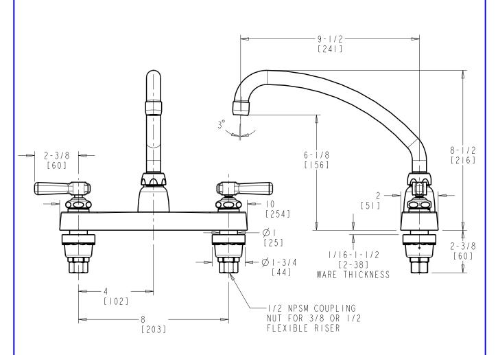
DIMENSIONS ARE IN INCHES AND [MILLIMETERS].
