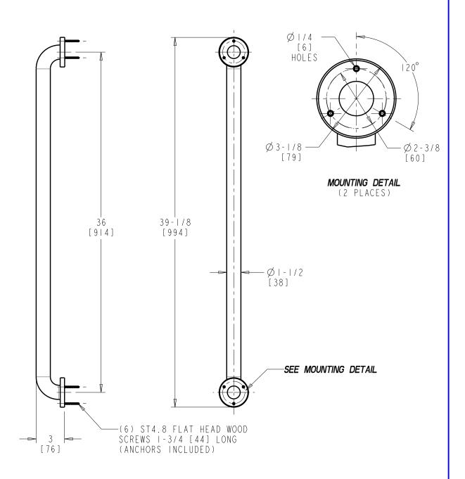
DIMENSIONS ARE IN INCHES AND [MILLIMETERS].
