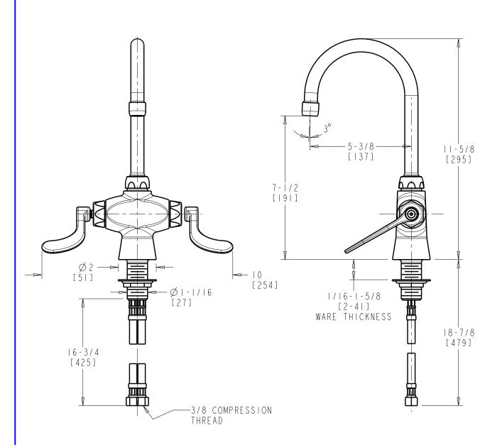
DIMENSIONS ARE IN INCHES AND [MILLIMETERS].
