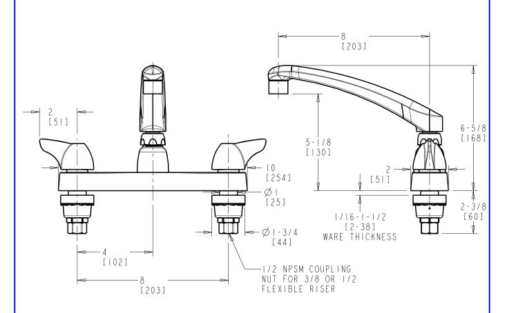
DIMENSIONS ARE IN INCHES AND [MILLIMETERS].
