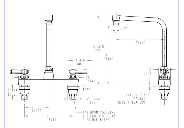
DIMENSIONS ARE IN INCHES AND [MILLIMETERS].
