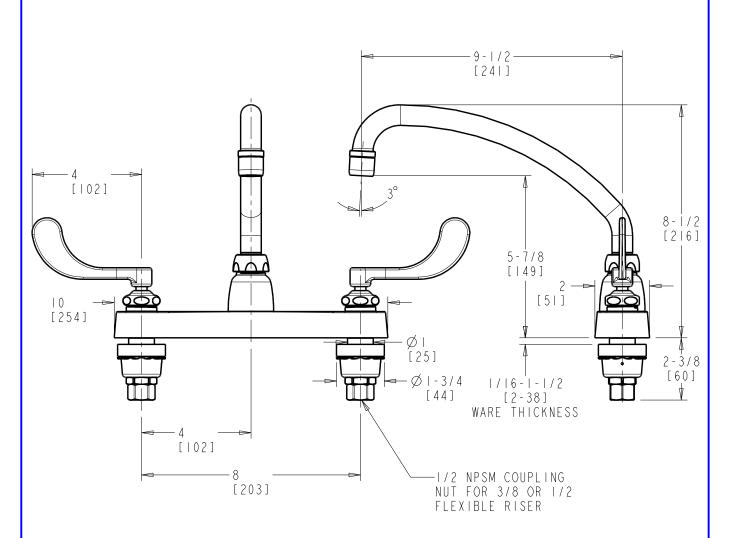
DIMENSIONS ARE IN INCHES AND [MILLIMETERS].
