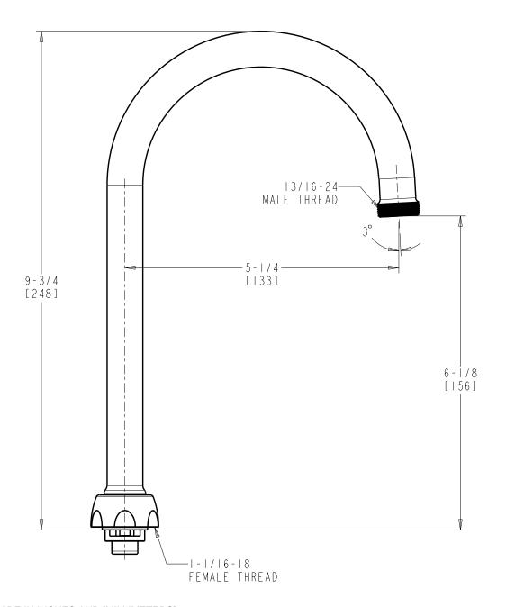
DIMENSIONS ARE IN INCHES AND [MILLIMETERS].
