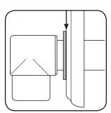
5. Push seal inside the drain back opening until it seats flush against the drain body.
