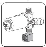
1. Install valve with brazed elbow
