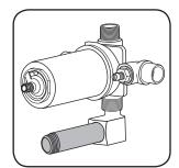
2. Install straight nipple 1/2" pipe – 1/2-14 NPT both ends. Use pipe sealer on both ends of pipe nipple. Tighten securely with wrench. Take care not to damage chrome plate finish.
