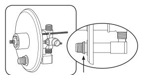
3. Position 2-hole round trim over valve and pipe and attach with screws. Insert pipe and drain seal with larger diameter end closest to the trim.
