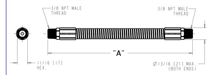
DIMENSIONS ARE IN INCHES AND [MILLIMETERS].
