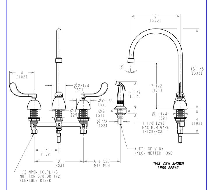
DIMENSIONS ARE IN INCHES AND [MILLIMETERS].
