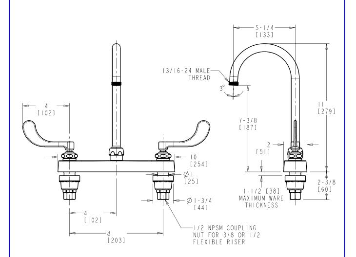
DIMENSIONS ARE IN INCHES AND [MILLIMETERS].
