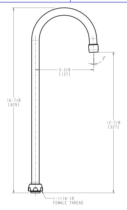
DIMENSIONS ARE IN INCHES AND [MILLIMETERS].
