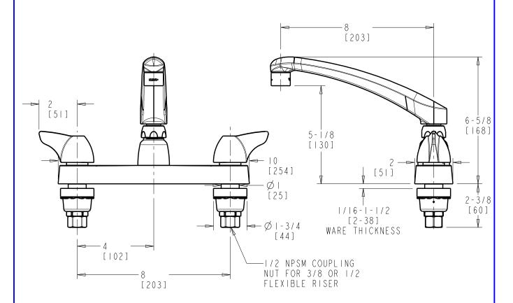
DIMENSIONS ARE IN INCHES AND [MILLIMETERS].
