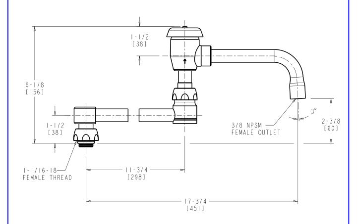
DIMENSIONS ARE IN INCHES AND [MILLIMETERS].
