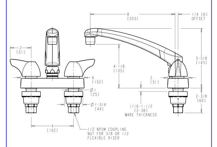
DIMENSIONS ARE IN INCHES AND [MILLIMETERS].
