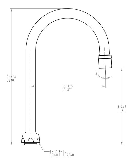
DIMENSIONS ARE IN INCHES AND [MILLIMETERS].
