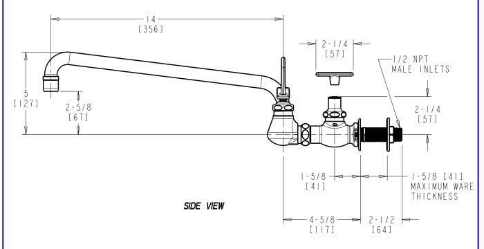
DIMENSIONS ARE IN INCHES AND [MILLIMETERS].
