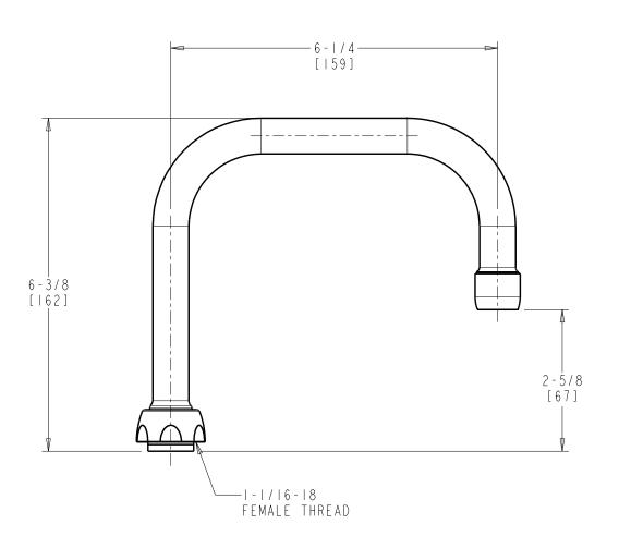
DIMENSIONS ARE IN INCHES AND [MILLIMETERS].
