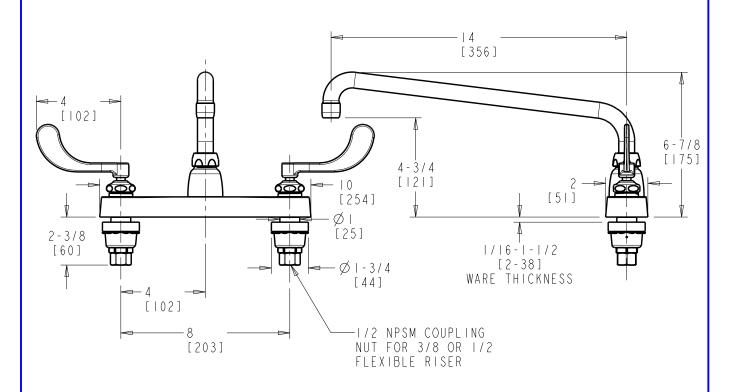
DIMENSIONS ARE IN INCHES AND [MILLIMETERS].
