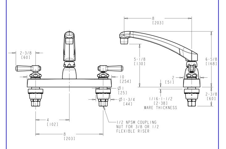
DIMENSIONS ARE IN INCHES AND [MILLIMETERS].
