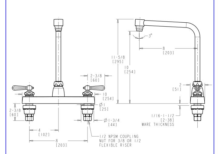
DIMENSIONS ARE IN INCHES AND [MILLIMETERS].
