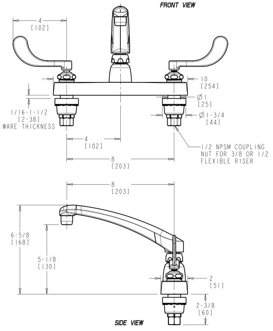
DIMENSIONS ARE IN INCHES AND [MILLIMETERS].
