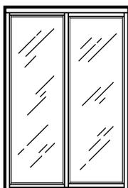
**General:** Furnish and install as shown on plans, a STYLEMATE® By-Pass enclosure as manufactured by E.L. Mustee & Sons, Inc. Model \_\_\_\_\_ with a bright (Chrome, Brushed Nickel, Oil-Rubbed Bronze) finish. Shall be by-pass style with aluminum frame and clear tempered safety glass panel. Continuous pull handle. Out-of-plumb condition up to 1" can be adjusted. Shall meet ANSI Specifications Z97.1
