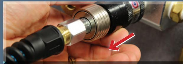
Black sleeve is pulled down to start air flow.
