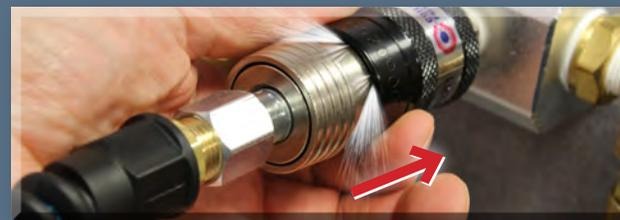
Black sleeve is pushed up to stop air flow and safely vent downstream pressure.
