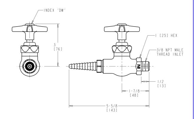
DIMENSIONS ARE IN INCHES AND [MILLIMETERS].
