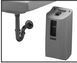
4. Position the enclosure against the wall. Ensure the tubing assembly and power cable from the spout will reach the bottom of the enclosure.
