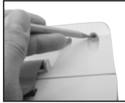
5. Mark the three mounting holes with a pencil (2 on the top and 1 on the bottom).
