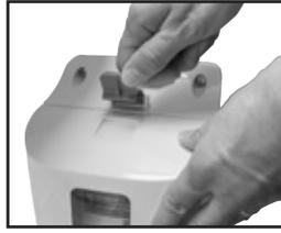
1. To open the enclosure, lift the blue cover latch. A hardware bag and tubing assembly are inside the enclosure.
