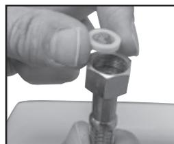
1. With the mixing valve installed, insert filter into the nut of stainless steel EFS supply hose. Connect and tighten to the outlet port of the tempering valve. Open the supply stops and check for leaks.
