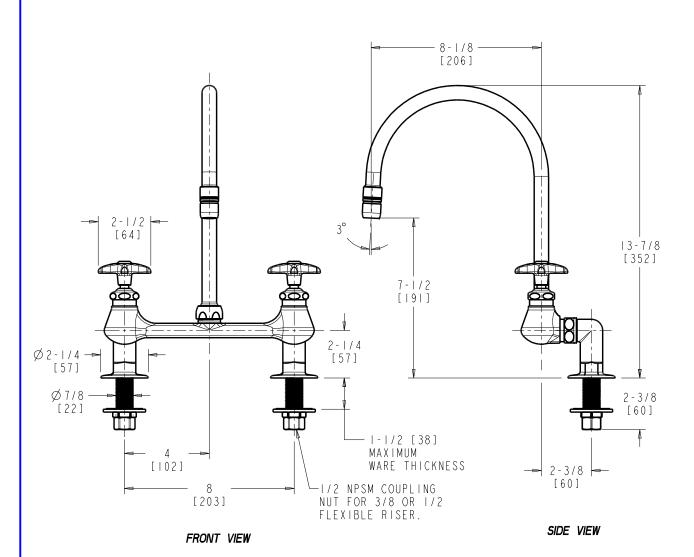
DIMENSIONS ARE IN INCHES AND [MILLIMETERS].
