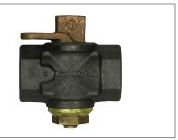
Cast iron body, brass plug manually operated 175 PSIG natural, manufactured, or propane gas valve for use in above ground gas piping systems in ambient temperatures between -20°F to 150°F. Iron body valves considered full port of flow. Made in the USA.
