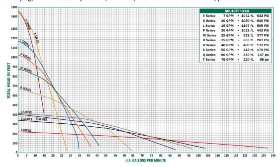
NOTE: Performance shown does not include friction loss in drop pipe (for flow rates above 25 GPM, larger drop pipe is recommended.)
