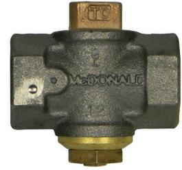
Cast iron body, brass plug manually operated 175 PSIG natural, manufactured, or propane gas valve for use in above ground gas piping systems in ambient temperatures between -20°F to 150°F. Iron body valves considered full port of flow.
