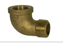
A.Y. M<sup>o</sup>Donald Mfg. Co. No-Lead Pipe Fittings & Nipples are constructed from heavy duty bronze and are rated for commerical, industrial and residential applications up to 125 WOG. Threads conform to ANSI B1.20.1 and fitting dimensions comply with ANSI B16.15.
