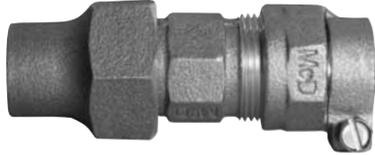
A.Y. McDonald Service Fittings are made in the United States of America and are manufactured to meet or exceed the AWWA C800 (latest revision) standard. Our service fittings are rated to withstand the same pressures as the tubing they are designed to fit. They are designed and tested for cold potable water **only**. EPDM rubber gaskets are used in our compression fittings.
