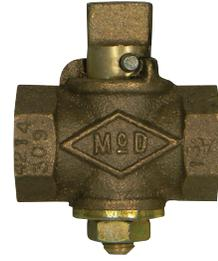
Bronze body and plug manually operated low pressure natural or propane gas valve for use indoors on house piping system between the meter outlet and the inlet connection of the gas appliance at ambient temperatures of 32 to 125 degrees Fahrenheit.
