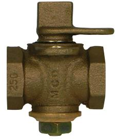
Brass body and plug manually operated low pressure natural or propane gas valve for use indoors on house piping system between the meter outlet and the inlet connection of the gas appliance at ambient temperatures of 32 to 125 degrees Fahrenheit.
