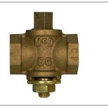
Brass body and plug manually operated low pressure natural or propane gas valve for use indoors on house piping system between the meter oulet and the inlet connection of the gas appliance at ambient temperatures of 32 to 125 degrees Fahrenheit.
