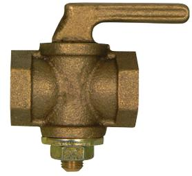
Brass body and plug manually operated low pressure natural or propane gas valve for use indoors on house piping system between the meter outlet and the inlet connection of the gas appliance at ambient temperatures of 32 to 125 degrees Fahrenheit.
