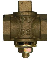
Bronze body and plug manually operated low pressure natural or propane gas valve for use indoors on house piping system between the meter outlet and the inlet connection of the gas appliance at ambient temperatures of 32 to 125 degrees Fahrenheit.
