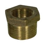
A.Y. M<sup>o</sup>Donald Mfg. Co. No-Lead Pipe Fittings & Nipples are constructed from heavy duty brass and are rated for commerical, industrial and residential applications up to 125 WOG. Threads conform to ANSI B1.20.1 and fitting dimensions comply with ANSI B16.15.
